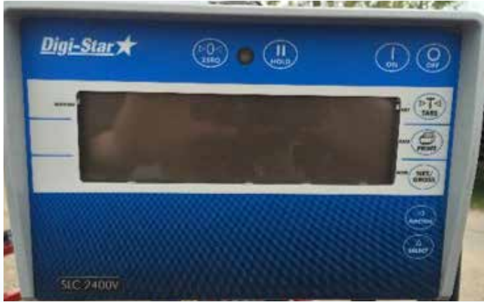
Bulk-Fill Weigh Scale for Monitoring Seed Tank Level
