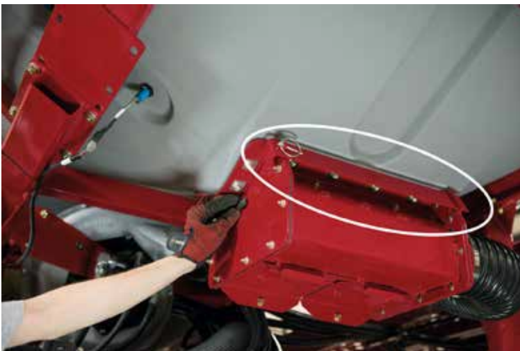
Blockoff Plate Stored
